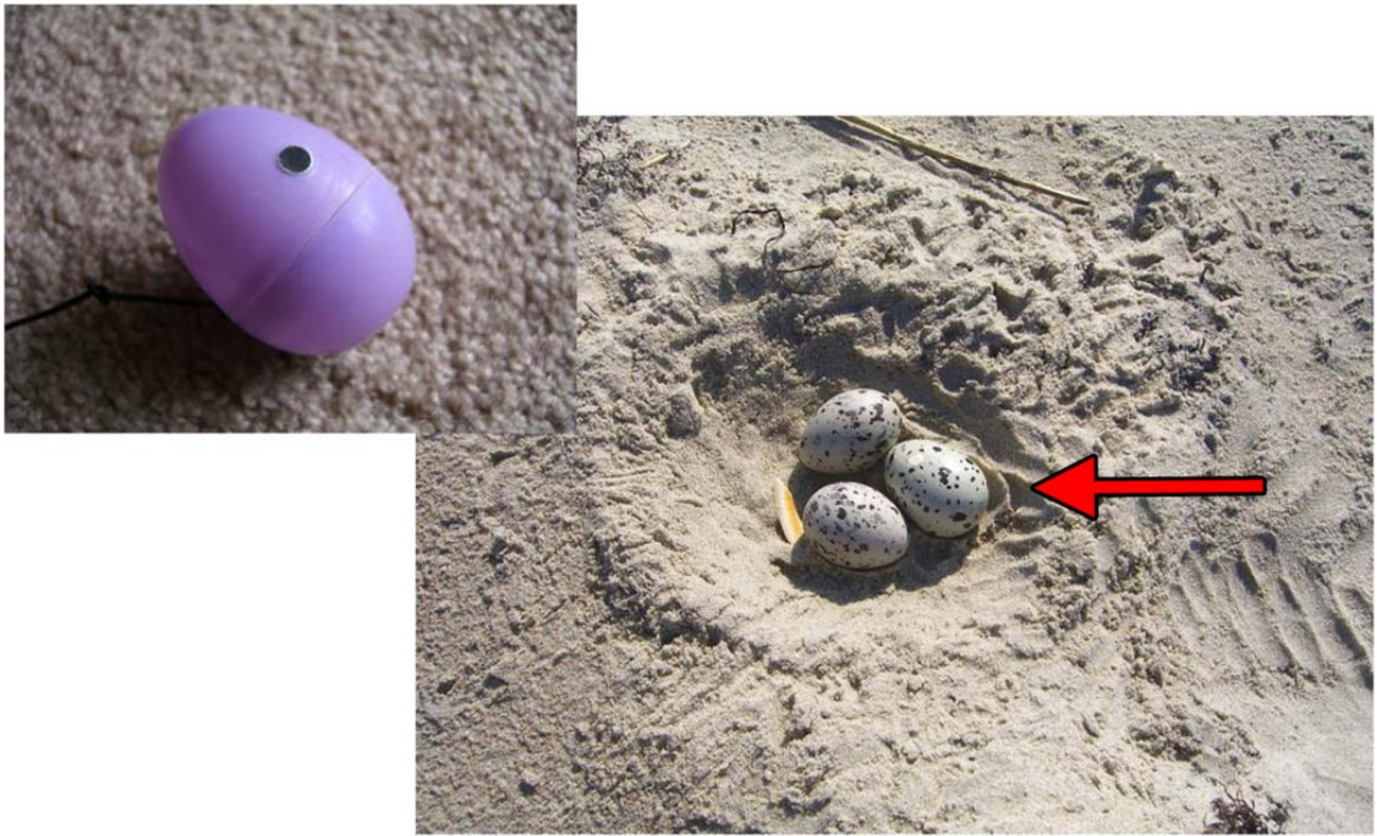
Figure 6. A plastic egg with an embedded microphone (left). Once covered and painted to resemble real American Oystercatcher eggs, the sensors were added to an active nest and used to record the heart rate of incubating American Oystercatchers (right). The red arrow indicates the artificial egg in the nest.
