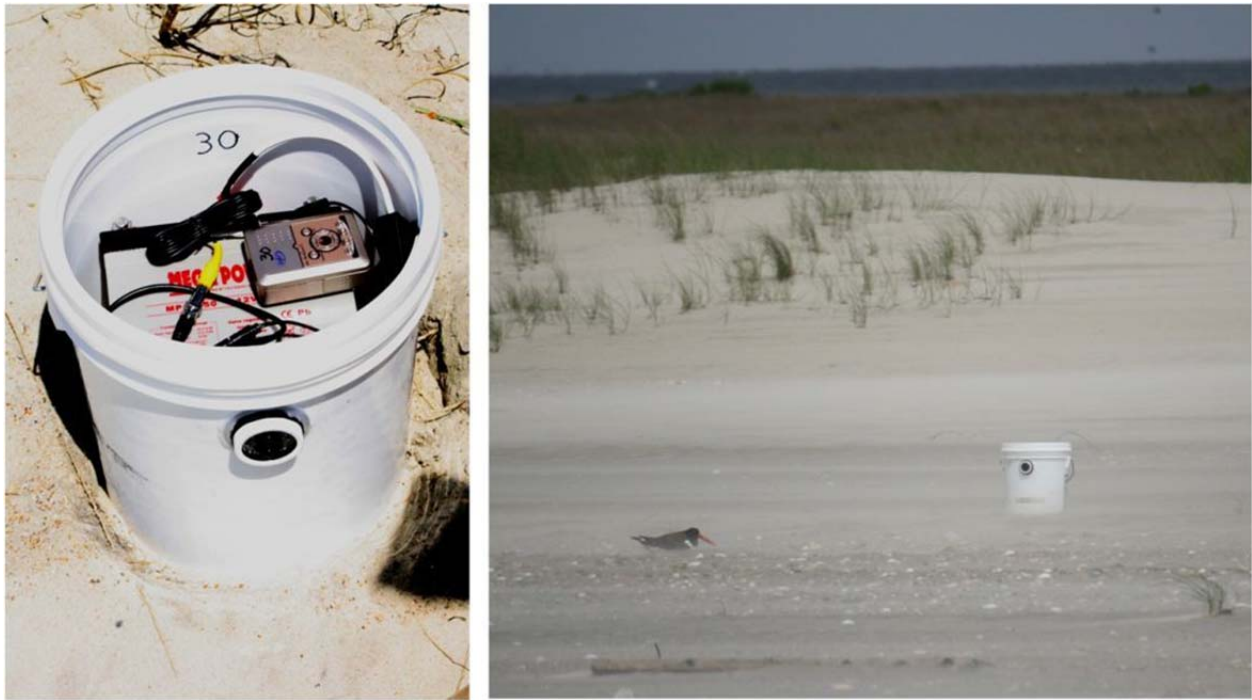
Figure 5. Camera unit for video recording incubating American Oystercatchers at nests. The recording system consisted of a camera, digital video recorder, and batteries encased in a white 5-gallon plastic bucket (left). A camera unit in action recording an incubating oystercatcher (right).
